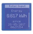
ePDU G3 provides one percent revenue-grade power monitoring for higher accuracy in department billing or colocation data centers. Effectively measure power usage to all outlets or individual outlets.
