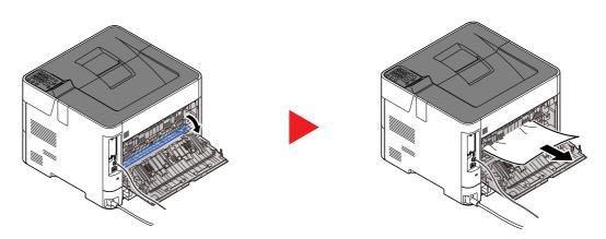
If you cannot find a paper jam, try checking inside the rear of the machine.
