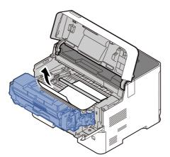
If the jammed paper appears to be pinched by rollers, pull it along the normal running direction of the paper.
