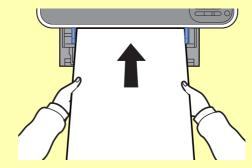
• After printing starts, catch the paper when it is output so that it does not fall. When using the inner tray as the output location, do not stand up the stopper.
