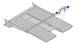
3 Install the rear tray on the rear of the machine.
