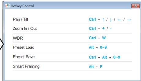
A hotkey tip will display when mouse is moved to the PTZ control button in PTZ mode.
