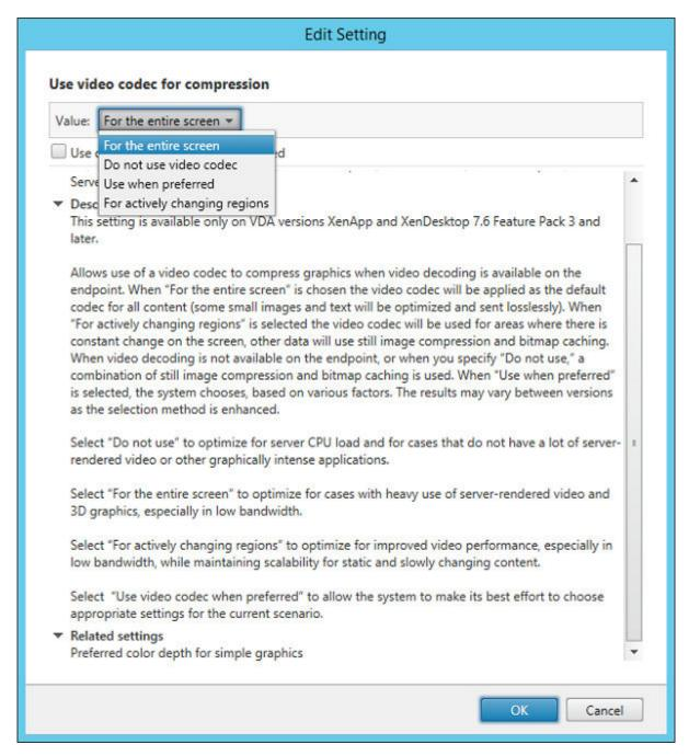
Figure 19. Use video codec for compression setting
