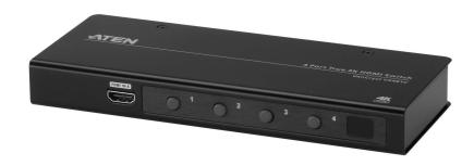
The ATEN VS481C is designed for applications that require the routing of 4 sources to one compatible display device. It enables the reliable transmission at video resolutions up to True 4K (4096 x 2160 @ 60Hz 4:4:4), data rates up to 18 Gbps, 3D, Deep Color up to 12-bit, and HD lossless audio formats. Integrator-friendly features include Auto Switching modes for auto port selection, bi-directional RS-232, and IR for remote device control.
