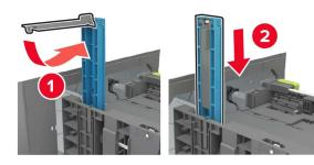
**d** Squeeze, and then slide the length guide to the correct position for the size of the paper being loaded.
