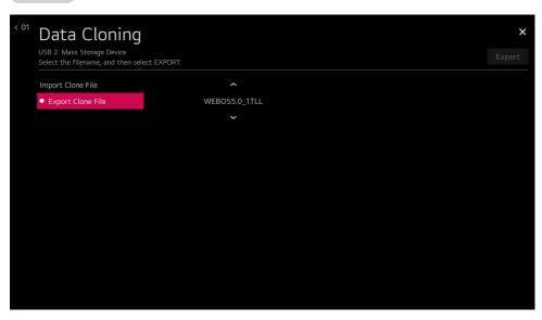
• "Export Clone File" creates "TLL" file in USB root folder. "TLL" file can be used to "Import Clone File". While writing is in process, the user must not turn STB off nor unplug the USB memory card. The following reference images might be slightly different.
