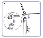
Put the stand base onto the stand neck as the direction shown in the figure. Check that the stand neck is firmly connected.
