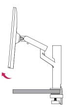
3 Rotate the monitor counter-clockwise as shown in the figure.
