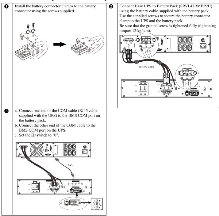
**NOTE 1 :** SRVL48RMBP2U can only be used with SRVL series, 1000VA, 2000VA and 3000VA Easy UPS. **NOTE 2 :** The above illustrations are shown for 1000VA UPS. The same procedures are applicable for both 2000VA and 3000VA UPS.
