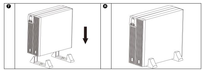
NOTE: Maintain approximately 70 mm distance from the edge of the unit, when installing the stabilizer brackets to the Easy UPS.
