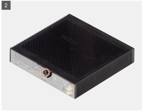
1. Align the tabs on the side cover with the slots on the chassis.
