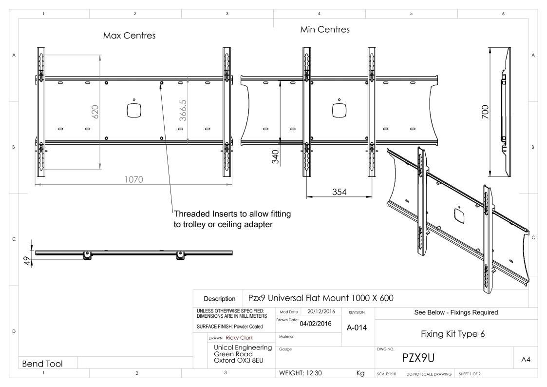
3 2 5 6 All Fixings must be approved by a builder or architect and these are only shown for illustrational purposes Ensure that the walls the load - (screen including all bracketry and peripherals).
