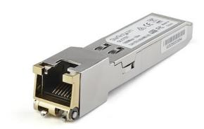
The RXGETSFPST is a Juniper RX-GET-SFP compatible copper transceiver module that has been designed, programmed and tested to work with Juniper brand switches and routers. It delivers dependable 1 GbE connectivity over copper cable, for 1000BASE-T compliant networks, with a maximum distance of up to 100 m (328 ft).
