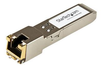
The 95Y0549-ST is a Brocade 95Y0549 compatible copper transceiver module that has been designed, programmed and tested to work with Brocade brand switches and routers. It delivers dependable 1 GbE connectivity over copper cable, for 10/100/1000 compliant networks, with a maximum distance of up to 100 m (328 ft).
