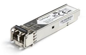
The SFP1GSXEMCST is a Dell EMC SFP-1G-SX compatible fiber transceiver module that has been designed, programmed and tested to work with Dell EMC brand switches and routers. It delivers dependable 1 GbE connectivity over fiber cable, for 1000BASE-SX compliant networks, with a maximum distance of up to 500 m (1640 ft)).
