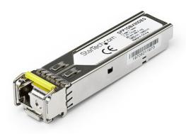
The SFP1GBX80DES is a Dell EMC SFP-1G-BX80-D compatible downstream fiber SFP transceiver which pairs with StarTech.com's SFP1GBX80UES. They are designed, programmed and tested to work with 1000BASE-BX80 compatible Dell EMC switches and routers. The SFP transceiver module supports a maximum distance of up to 80 km (49.7 mi) and delivers dependable 1 GbE connectivity over fiber cabling.
