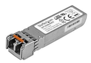
The SFP10GBLRMST is an MSA compliant fiber SFP transceiver that's designed, programmed and tested to work with 10GBASE-LRM compatible MSA switches and routers. The SFP+ transceiver module supports a maximum distance of up to 220 m (721 ft.) and delivers dependable 10 GbE connectivity over fiber cabling. <br/>
