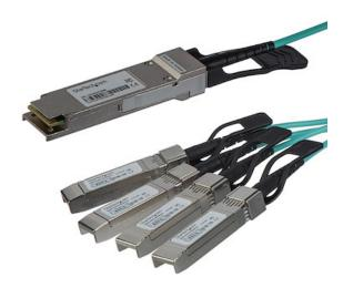
The QSFP4X10GAO3 is a Cisco QSFP-4X10G-AOC3M compatible optical quad small form-factor pluggable (QSFP+) breakout cable that is designed, programmed and tested to work with Cisco brand compatible servers or routers and complies with MSA industry standards. Connecting a single QSFP+ port (40 GbE) to four 10G SFP+ ports, this active optical breakout cable is fully hot-pluggable which makes upgrades and replacements seamless by minimizing network disruptions.
