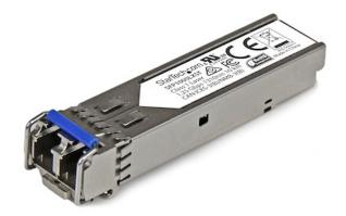
The SFP1000LXST is an MSA compliant fiber SFP transceiver that's designed, programmed and tested to work with 1000BASE-LX compatible MSA switches and routers. The SFP transceiver module supports a maximum distance of up to 10 km (6.2 mi) and delivers dependable 1 GbE connectivity over fiber cabling. <br/> <br/>
