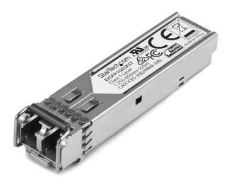
The EXSFP1GESXST is a Juniper EX-SFP-1GE-SX compatible fiber transceiver module that has been designed, programmed and tested to work with Juniper brand switches and routers. It delivers dependable 1GbE connectivity over fiber cable, for 1000BASE-SX compliant networks, with a maximum distance of up to 550 m (1804 ft).
