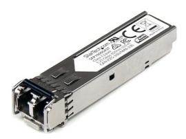
The SFP1000SXST is an MSA compliant fiber SFP transceiver that's designed, programmed and tested to work with 1000BASE-SX compatible MSA switches and routers. The SFP transceiver module supports a maximum distance of up to 550 m (1804 ft) and delivers dependable 1 GbE connectivity over fiber cabling. <br/>
