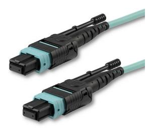
This MPO/MTP fiber optic cable houses 12 fibers and lets you interface between different networking devices of varying speeds. For example, you can set up a one-to-one connection between two 40Gbps switches or servers. Alternatively, you can connect a 40Gbps switch and break out the 40Gbps into six duplex 10Gbps LC connections on a patch panel or network cassette, which then fans out to individual 10Gbps devices.
