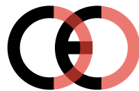
False CE Mark (too close)
