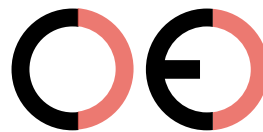
False CE Mark (too far)
