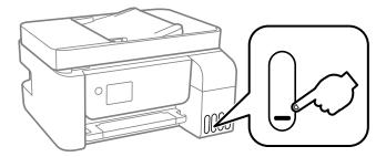
**Note:** The product has a low ink alert system. The accuracy of this system depends on the user refilling the ink tanks correctly. The product cannot directly measure the ink levels in the tanks; instead it estimates the amount of ink remaining by internally monitoring ink usage. The low ink alert system may generate inaccurate messages if the ink tanks are not refilled according to these instructions.
