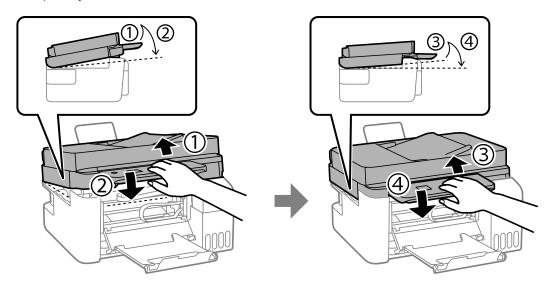
Note: The scanner unit must be closed completely before it can be opened again.
