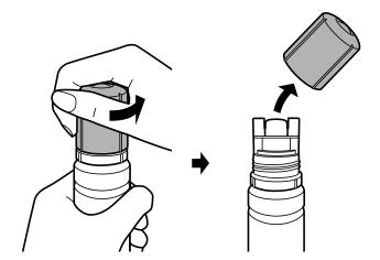
**Caution:** Do not shake or squeeze the bottle. Do not touch the top of the bottle after its cap is removed. Do not allow the top of the ink bottle to hit any objects after removing its cap; otherwise, ink may spill.
