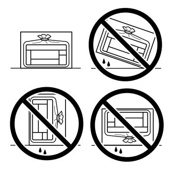
• When storing or transporting an ink bottle after removing its seal, do not tilt the bottle and do not subject it to impacts or temperature changes. Otherwise, ink may leak even if the cap on the ink bottle is tightened securely. Be sure to keep the ink bottle upright when tightening the cap, and take measures to prevent ink from leaking when transporting the ink bottles.
