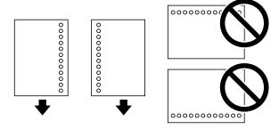
• To load a sheet of paper longer than legal size, close the paper support, then load the leading edge of the paper as shown.
