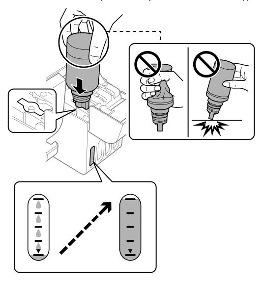
**Note:** If ink does not flow from the bottle, lift and reinsert the bottle. If the ink has reached the upper line of the tank, do not remove and reinsert the bottle or ink may leak.
