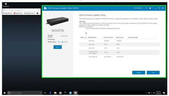
e. Wait for all the component firmware update to complete. A progress bar is displayed in the bottom.
