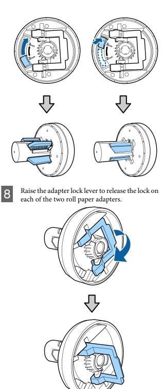
9 Attach the roll paper adapters to both ends of the roll paper, and then lower the lock levers on the left and right to lock them in place.
