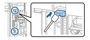
(4) If there is any fluff or dust in the caps, remove it with the tip of the cleaning stick or with tweezers.
