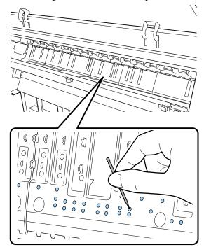
5 Use a commercially available cotton swab to wipe off the paper particles and dust from the inner edges of the pads for borderless printing as shown below.
