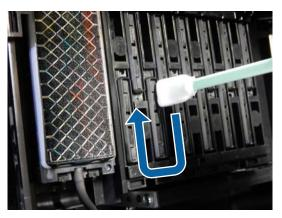
(2) Hold the cleaning stick so that it is vertical, and wipe the outer areas of all of the drying caps.
