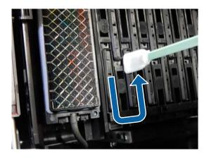
(3) Flatten the cleaning stick and wipe all of the edges of the drying caps.
