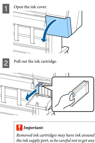
Removed ink cartridges may have ink around the ink supply port, so be careful not to get any ink on the surrounding area when removing the cartridges.
