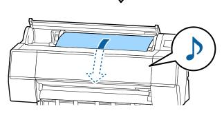
16 When auto paper feed is set to Off, insert the leading edge of the roll paper into the paper feed slot, and feed until the leading edge extends out of the printer.
