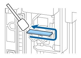
(3) Wipe any dirt off the upper edge of the wiper (three parts).
