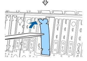
Press the pad for borderless printing into the pad section.
