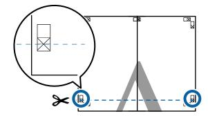
Lay the upper sheet on top of the lower sheet. Lineup the X marks as shown in the illustration below, and temporarily fasten them using an adhesive tape on the back.
