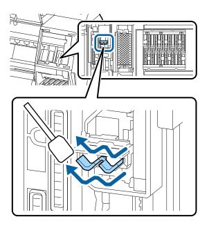
(2) Wipe any dirt off the outer edges of the wiper (one part).
