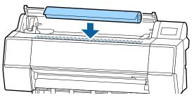
Adjust the size of the roll paper adapters to the size of the roll core.
