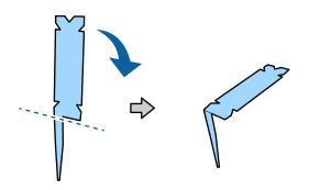
Bend the pad for borderless printing marked with an \* in the "Consumables and Options" illustration as shown in the diagram.
