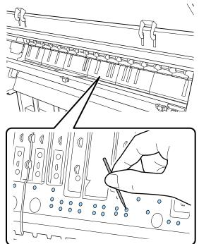
6 Remove paper particles and dust around the outer edges with commercially available cotton swabs as shown below.
