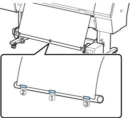
6 Flip the Manual switch on the auto take-up reel unit to Forward, and take up as much paper as possible.
