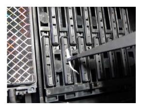
Use a new cleaning stick to wipe any dirt off the wipers (x 3).
