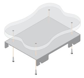
6. Slide the switch into the ceiling mount tray.
