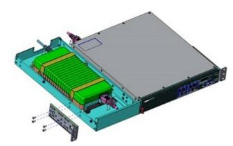
8. Install the L-bracket to the two-post rack, and secure it with the rack-mounting screws.
