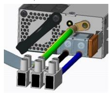
7. Attach the yellow and green wire to the PSU GND. Secure the wire with the M5 screw.
