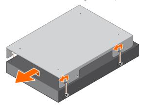
7. Line up the two mushroom-heads on the switch to the ceiling mount tray hook cutouts until the switch locks into place.
