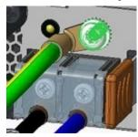
NOTE: To uninstall the cable from the 1300W DC PSU, remove the plastic cover and unscrew the M4 and M5 screws. Pull the 1300W DC cable out from the 1300W DC PSU socket.
