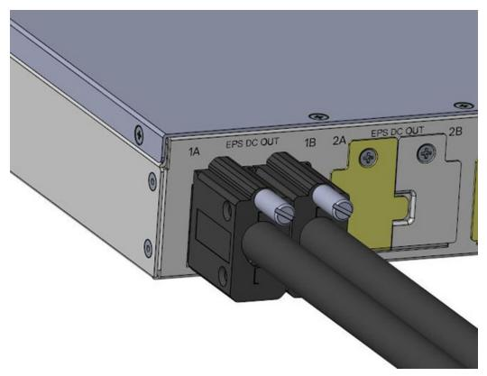
$\textbf{5.} \ \ \text{Repeat until all EPS power cables are connected}.$
