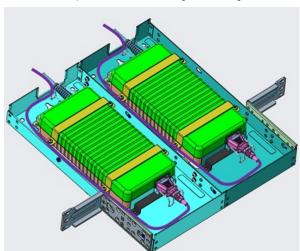
**9.** Install the dual-EPA assembly above the switch in the two-post rack. For rack installation instructions, see N3200-ON Series switch installation.
