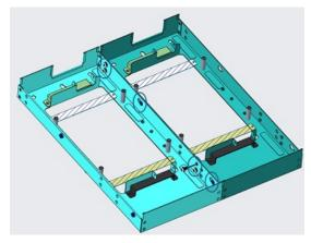
**3.** Install the two EPAs in your power adapter assembly and secure with metal straps and screws. For EPA installation instructions, see Power adapter holder assembly.
