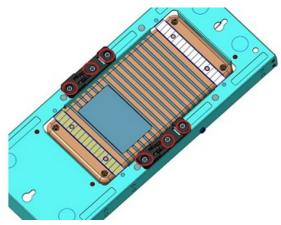
4. Snap the two DIN buckles into the DIN rails.
