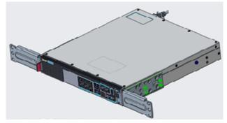
• For a center-mount installation, the standard bracket ears face the PSU-side of the switch.
