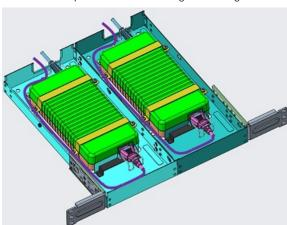
**9.** Install the dual-EPA assembly above the switch in the two-post rack. For rack installation instructions, see N3200-ON Series switch installation.
