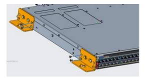
**3.** Repeat to attach two brackets to the right side of the switch.
