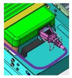
6. Install the four-post rail-brackets to the switch and the power adapter holder.
