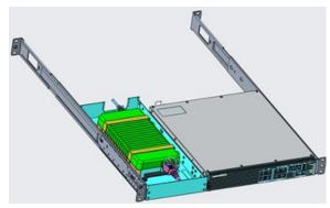
7. Install the rail bracket to the four-post rack and secure it with the rack-mounting screws.
