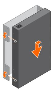
7. Line up the two mushroom-heads on the switch to the wall mount tray hook cutouts until the switch locks into place.
