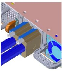
**4.** Connect the other end of the DC cable to either a MPS-1S shelf or MPS-3S shelf.
