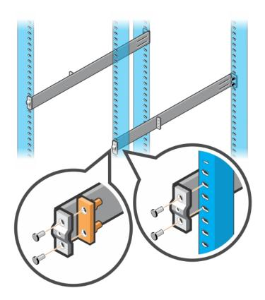
Figure 3. Four-post threaded round-hole installation
