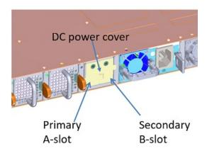
NOTE: If you are connecting a single EPS power cable to your switch, always use primary A-slot. Leave the secondary B-slot DC power cover in place, as shown:
