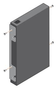
To uninstall the switch, unscrew the four wall mount tray screws and slide the switch from the mushroom head hooks.
