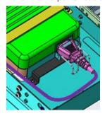
6. Secure the wire clip over the EPA cable.
