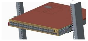
To uninstall the switch from the rack, unscrew the four #12-24 rackmount screws and slide the switch from the rack.
