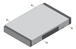
To uninstall the switch, unscrew the four ceiling mount tray screws and slide the switch from the mushroom head hooks.
