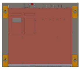
**9.** Screw the remaining four M5 screws into the anchors and tighten the screws. Torque the screws to 24 in-lbs.
