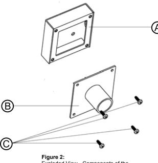
Exploded View - Components of the Ceiling Pendant Mount Kit
