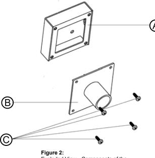
Exploded View - Components of the Ceiling Pendant Mount Kit
