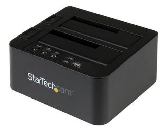
Duplicate drives quickly, at rates of up to 28GB per minute for SSDs, without having to connect to your computer. This duplicator dock offers standalone drive cloning that makes it easy to back up your data and make exact images of your drives. You can also connect the dock to your computer through USB 3.2 Gen 2 (10Gbps), to dock and swap your drives as part of a scalable storage solution.
