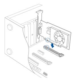
5. The ejector will snap back into place automatically.
