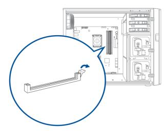
6. Align the notch on the bottom edge of the DIMM with the key of the DIMM socket, and then firmly insert the DIMM into the socket until the ejector snaps back into place.
