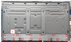
Use a screwdriver to remove10pcs screws for unlocking the two VESA brackets with back bracket.(Torque: 5±0.5kgf)
