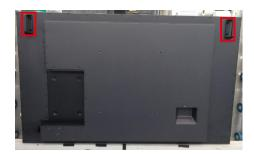
Remove the handles and rear cover, then use a screwdriver to remove 7pcs screws for releasing the PC box.(Torque: 4.5±0.3kgf)
