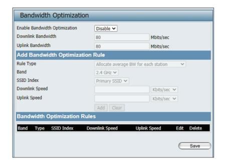
Band: Use the drop-down menu to toggle the wireless band between 2.4GHz and 5GHz.
