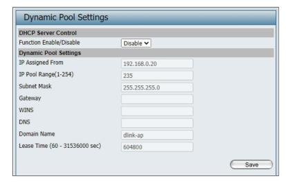
Subnet Mask: All devices in the network must have the same subnet mask to communicate. Enter the subnet mask for the network here.
