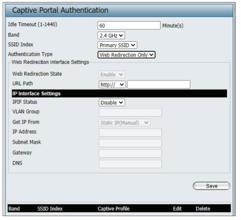
Static IP (Manual) is chosen here. Choose this option if you do not have a DHCP server in your network, or if you wish to assign a static IP address to the DAP-X2810. When Dynamic IP (DHCP) is selected, the other fields here will be grayed out. Please allow about 2 minutes for the DHCP client to be functional once this selection is made.
