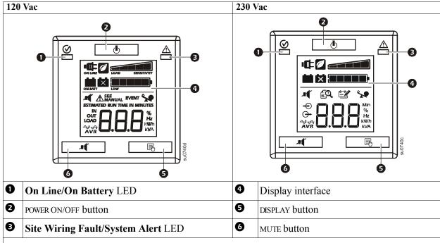
Note: Refer to "Feature Reference Guide" on page 10 in this manual for a detailed description of the front panel buttons and icons.
