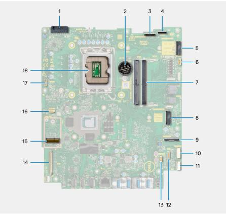
1. Power-supply unit (PSU) cable connector
