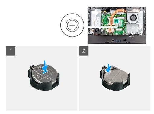
With the positive-side facing up, insert the coin-cell battery into the battery holder on the system board and gently press the battery until it snaps into place.
