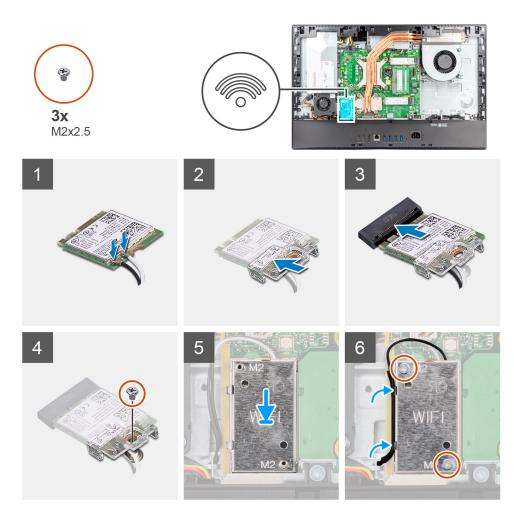
Connect the antenna cables to the wireless card. The following table provides the antenna-cable color scheme:
