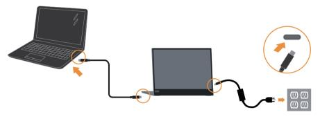
2) Connect Type-C power adapter to the left or right side of L15 and connect L15 to the mobile phone with a USB-C cable.
