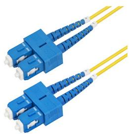
OS2 SC to SC Single Mode Duplex Fiber Optic Patch cable facilitates connectivity across 40G/100G networks. It supports Coarse Wavelength Division Multiplexing (CWDM) across an extended wavelength range of 1260-1625nm, improving channel isolation for optimal signal strength over long distances.
