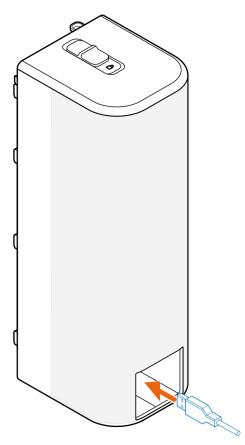
**3.** Connect the cables to their respective ports on the chassis.
