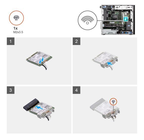
Connect the antenna cables to the WLAN card.
