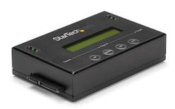
The SATDUP11 standalone hard drive duplicator eraser enables you to copy 1-to-1, or erase up to 2 SATA hard drives simultaneously without a host computer.
