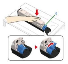
**13** Check the label color of the new image drum and place the drum into the machine.
