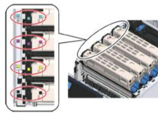
5 Turn the toner cartridge lock lever (blue) (5) of the toner cartridge toward you until its top align on the ▶ mark to detach the toner cartridge from the image drum.
