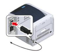
4 Insert one end of the USB cable into the USB interface connector on the machine.
