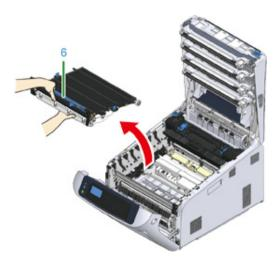
8 Hold the blue handle of a new belt unit, support the bottom of the belt unit, and insert the axis of the belt unit into the groove (7) in the printer.
