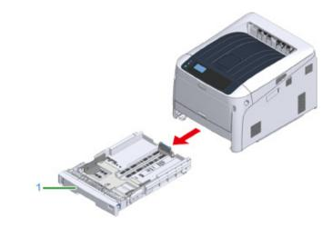
2 Set the paper size dial (2) to match the loading paper size. Set the dial to [A4] when loading the A4 size paper with a landscape orientation.
