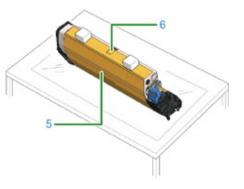
(2) Draw the protective sheet (5) in the direction of the arrow. Do not turn the toner cartridge lock lever (7) (blue).
