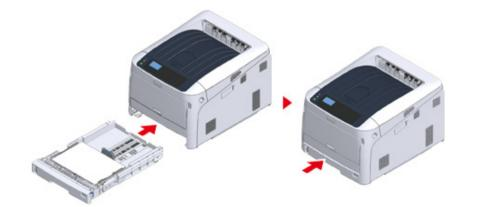
If using media that you cannot select the size with a paper size dial options, set the dial to [Other], and then set [Custom Size] on the operator panel and enter the width and length of paper.
