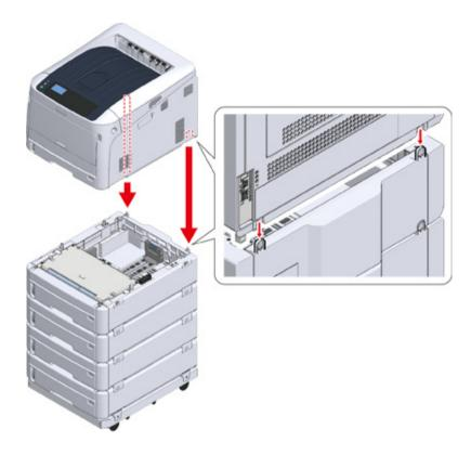
7 When attaching the additional tray unit, connect the printer unit and the additional tray unit.
