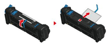
7 Pull the protective sheet in the direction of the arrow to remove.
