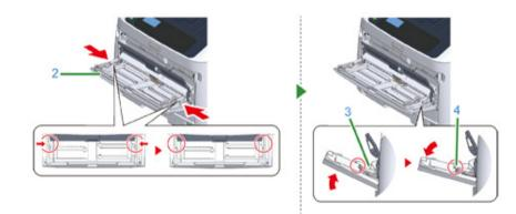
11 In the same manner, while pressing the left arm on the MP tray inward, slightly lift the MP tray and hook the tab.
