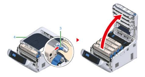
Identify the image drum to be replaced by its label color.
