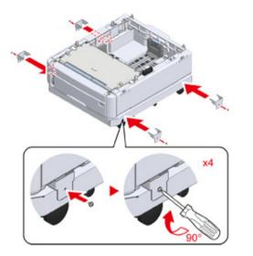
4 When adding on a further additional tray unit, gently place the unit on top so that the protrusions at the rear of the additional tray unit to be attached are
