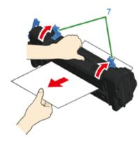
**9** If jammed paper remains in the machine, hold the both sides of the paper to remove it gently.
