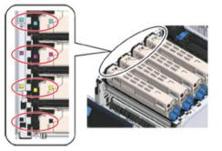
5 Remove the image drum (5) from the machine and place the image drum on a flat surface.
