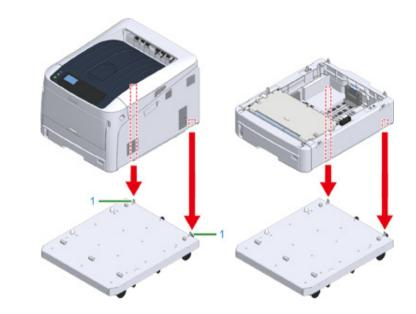
3 Connect the printer unit and the caster base or the additional tray unit and the caster base.
