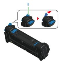
9 Hold the handle and place the new fuser unit into the machine.
