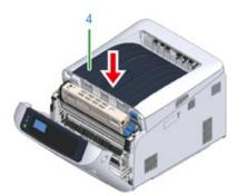
Close the front cover (2).Cannot close the front cover securely if the output tray is not closed.
