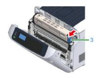
Lift the toner cartridge (4) from the right side, and remove it from the machine.
