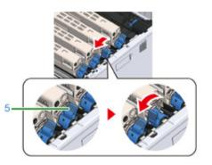
**6** Lift the toner cartridge (6) from right side, and remove it from the machine.
