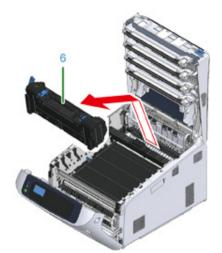
8 Lift the release levers (7) on the fuser unit, and pull out the jammed paper forward gently.
