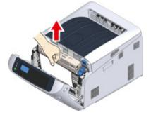
**3** Take out the duplex unit (3) by pulling it obliquely upward while holding the center recess on the back of the machine.
