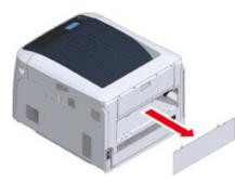
4 Ensure that the duplex unit is the right way up, as shown, and push it into the slot at the rear of the printer.
