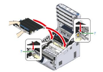
**9** Lower the handle side of the belt unit and set the belt unit to the machine.
