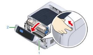
2 Remove the jammed paper gently in the direction of the arrow if an edge of jammed paper can be seen, and then go to step 8. If you cannot find jammed paper, go to step 3.
