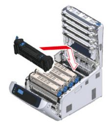
Push back the left locking lever (5) of the fuser unit to lock.
