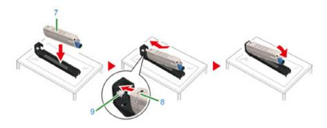
12 Turn the toner cartridge lock lever (blue) (6) of the toner cartridge backward until its top align on the ▶ mark while pressing the toner cartridge to attach the toner cartridge to the image drum.
