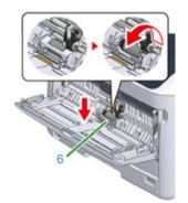
7 Wipe the separation rollers (7) with a wet cloth that has been wrung out well.
