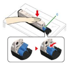
7 Lift the toner cartridge (7) from the right side, and remove it from the image drum.
