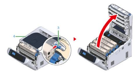
Identify the image drum to be replaced by its label color.
