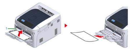
2 Insert your finger into the recess on the right side of the machine and pull the front cover open lever (2) to open the front cover (3) forward.
