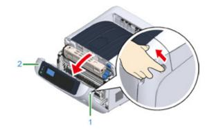
2 Remove the jammed paper gently in the direction of the arrow if an edge of jammed paper can be seen.
