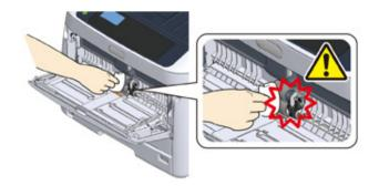
6 Open the separation roller cover (6) forward while pressing the center part of the MP tray.
