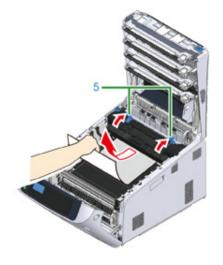
Return all four image drums into the machine carefully.
