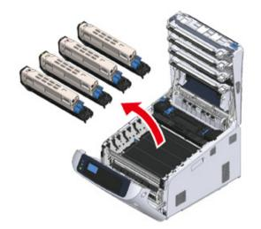
4 Cover the removed image drums with paper so that the image drums are not exposed to light.
