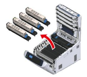
4 Cover the removed image drums with paper so that the image drums are not exposed to light.
