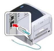
Insert the other end of the LAN (1) cable into the hub (2).
