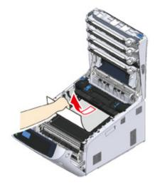
Pull out the jammed paper gently while lifting the release levers (5) on the fuser unit if an edge of jammed paper cannot be seen.
