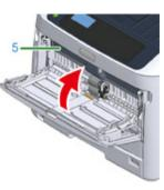
5 Wipe paper feed rollers with a wet cloth that has been wrung out well.
