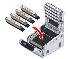
7 Close the output tray (4) by pushing the center of the cover firmly.
