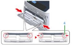
3 In the same manner, slightly lifting the MP tray, press the left arm inward, then unlock the tab.
