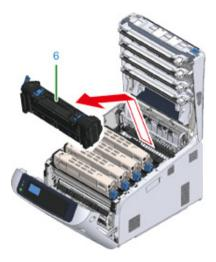
6 Peel off the tape from the new fuser unit, and pass the tape through the handle of the fuser unit.
