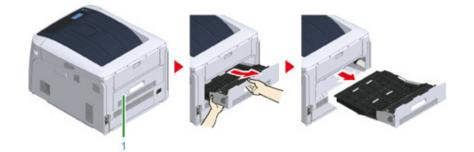
2 Check for jammed paper inside the machine. If jammed paper remains, remove it.
