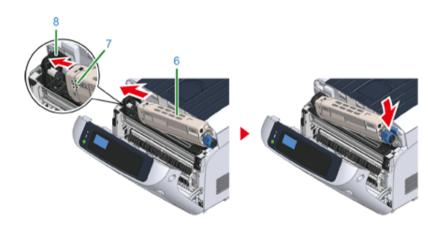
8 While pressing the toner cartridge, turn the toner cartridge lock lever (blue) (3) backward until its to aligns on the ▶ mark, and lock the toner cartridge to the image drum.
