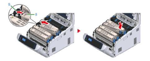
10 While pressing the toner cartridge, turn the toner cartridge lock lever (blue) (5) backward until its to aligns on the ▶ mark, and lock the toner cartridge to the image drum.
