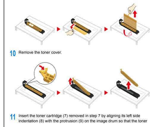
cartridge and image drum color label align. Then insert the right side gently into place.
