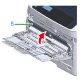
5 Adjust the manual feeding paper guide (6) to the width of paper to be loaded.
