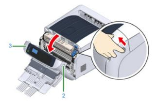
3 Remove the jammed paper gently by pulling the edge of paper.
