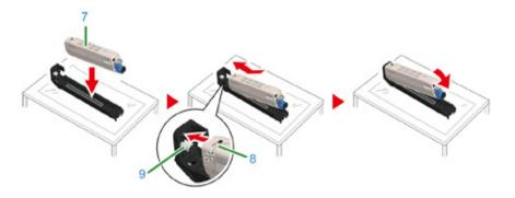
12 Turn the toner cartridge lock lever (blue) (10) of the toner cartridge backward until its top align on the ▶ mark while pressing the toner cartridge to attach the toner cartridge to the image drum.
