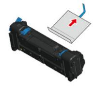
8 Pull forward the left locking lever (5) of the fuser unit.
