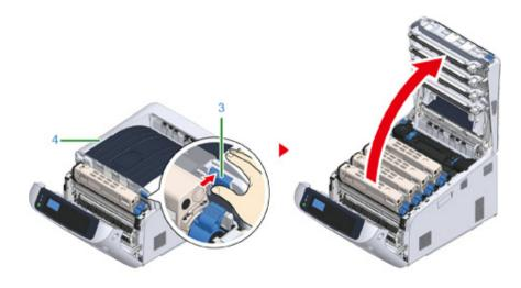
6 Hold the toner cartridge with both hands and pull it out along with the image drum. Pull out all 4 colors of toner cartridge and image drums, and set it on a flat surface covered with sheets of newspaper, etc.
