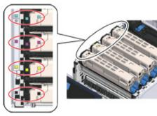
5 Remove the image drum (5) from the machine and place it on a flat surface.
