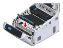
Turn the blue knobs (5) on both sides of the belt unit in the direction of the 10 arrow to lock the belt unit.
