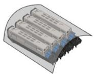
**6** Turn the blue knobs (5) on each side of the belt unit in direction of the arrow to unlock.
