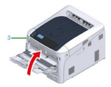
5 If loading paper on MP tray, lift the paper set cover (1) and set the paper with the print side face up.
