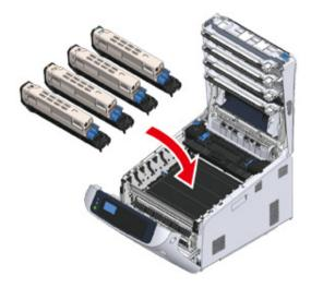
**13** Close the output tray (4) by pushing the center of the cover firmly.
