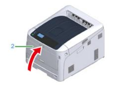
11 If optional additional tray units are installed, detach the parts connecting the machine and the additional tray units.
