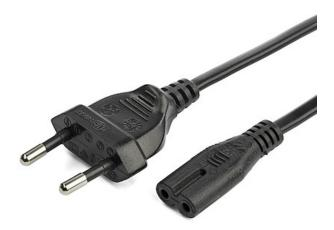
The 752E-2M-POWER-LEAD 2m Laptop Power Cord features one EU plug (CEE 7/16 Alternative II) and one non-polarized IEC 60320 C7 Connector It is a suitable replacement cable for a Lenovo, IBM, or other compatible laptop power bricks that features a C8 inlet.
