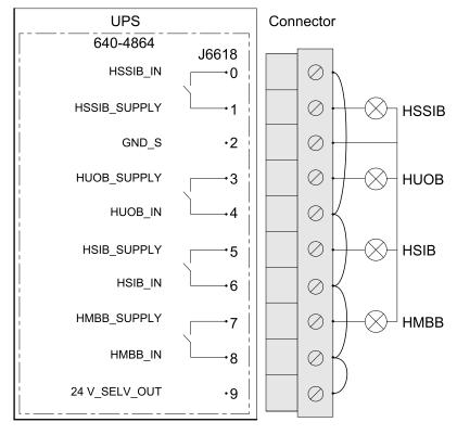
2. Connect signal cables from AUX switches in your switchgear to board 640-4843 in the top of the UPS.
