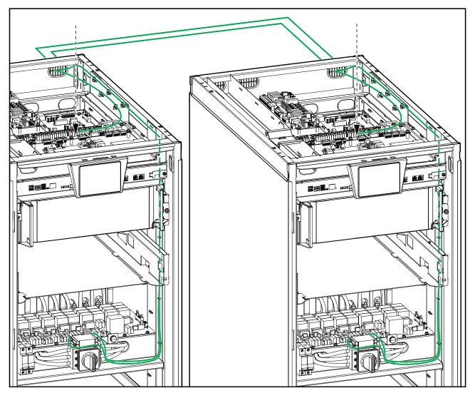
4. Reinstall the front cover and the static switch module on both UPSs.
