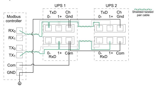
Install 150 Ohm termination resistors at each end of each bus if the buses are very long and operate at high data rates. Busses under 610 meters (2000 feet) at 9600 baud or under 305 meters (1000 feet) at 19.200 baud should not require termination resistors.
