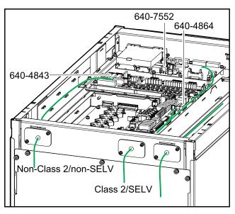
12. Remove the conduit box from the rear of the UPS.
