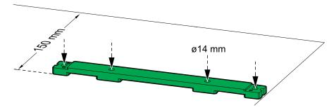
2. Install the rear anchoring bracket on the UPS with the provided M8 bolts.
