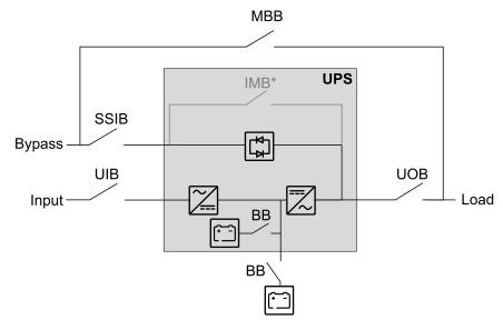
**NOTE:** The internal maintenance breaker IMB\* cannot be used in a system with an external maintenance bypass breaker MBB and the internal maintenance breaker IMB\* must be padlocked in the open position.
