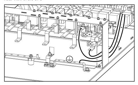
6. Route the PE cable and the DC cables into modular battery cabinet 1 and connect the PE cable and DC cables in modular battery cabinet 1.
