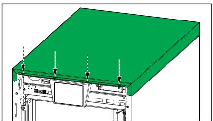
3. **Only for seismic anchoring**: Push the UPS into position so the rear anchoring bracket connects to the rear anchor.
