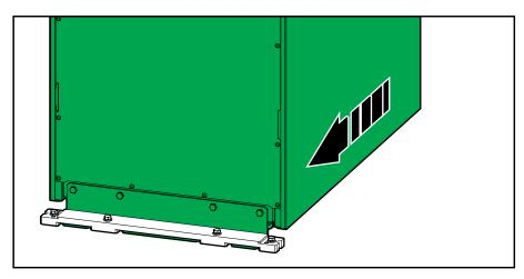
4. Lower the front and rear leveling feet on the UPS with a wrench until they connect with the floor. Use a bubble-leveler to check that the UPS is level.
