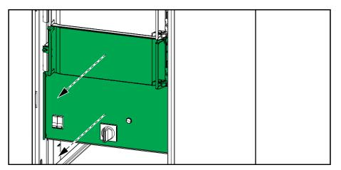
2. Install an additional AUX switch (provided) on the internal maintenance breaker IMB on both UPSs.
