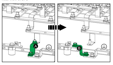
2. Remove the three single mains jumper busbars.
