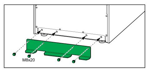
3. Install the seismic front anchoring bracket on the UPS with the provided M8 bolts.
