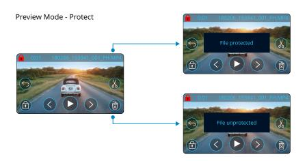
While in Preview Mode, press the Protect Button to protect/unprotect a file. When a file is protected, a red padlock icon will appear in the top left of the screen.
