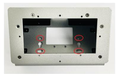
2 Remove the mounting plate from the Touch Panel and secure it onto the enclosure with the two M3x5 screws provided.
