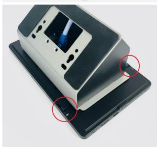
7 Secure the Touch Panel to the mounting plate with the screw you removed at step 2.
